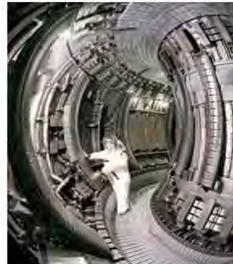
Beryllium worker wearing pressurized suit inside the Joint European Torus (JET) vessel
