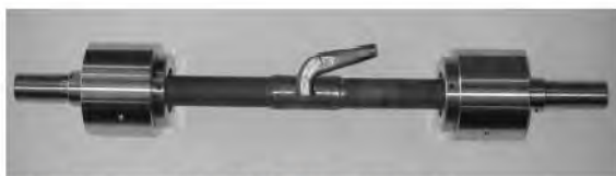
ITER Fatigue test at 4.2 K of TF coil He inlet
