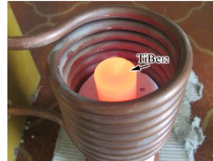
Induction heating of a \text{TiBe}_{12} sample
