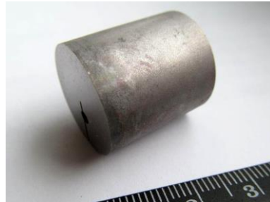
No cracks or severe oxidation observed after thermo-cycling
